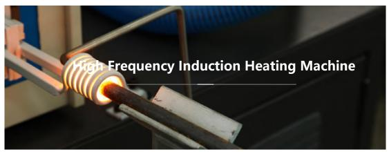
The working frequency of CX series high-frequency induction heating equipment covers 50KHZ ~ 120KHZ. It is widely used in induction welding, tool welding, pipe welding, thermal nesting, thermal packaging, etc.
